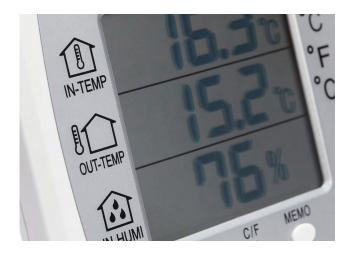
A hygrometer is an instrument used for measuring the moisture content in the atmosphere.
